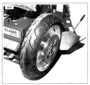
Figure 2-80. Pneumatic Bead Breaker
