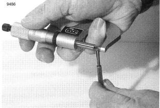
Figure 3-55. Measure Stem to Guide Clearance
