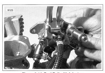
Figure 3-14. Fuel Rail with Injectors
