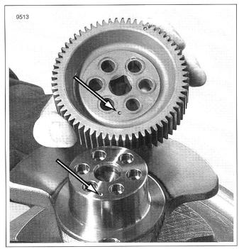
Figure 3-209. Primary Gear Timing Marks
