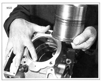
Figure 3-215. Clean Liner and Case Step
