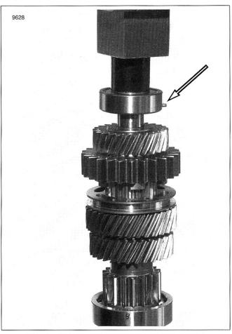
Figure 7-38. 2nd Gear Bearing Alignment Pin
