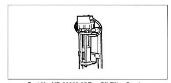
Part No. HD-39823 25 Ton Oil Filter Crusher
