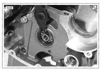
Figure 3-175. Outboard Retaining Ring Installation
